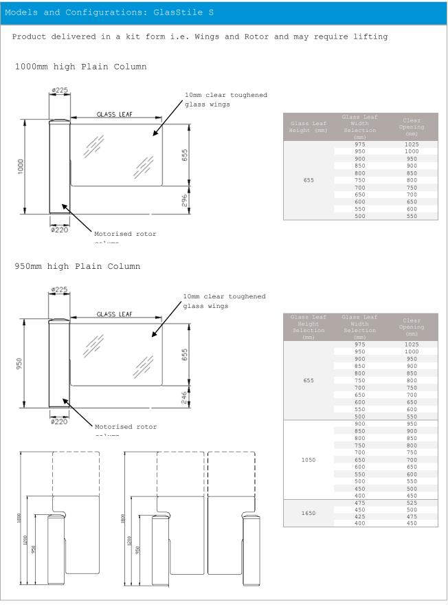
Concrete Base to specification at least fck (cube) 300N/mm2 of resistance. Base to be flat and level to +/- 5mm over footprint
